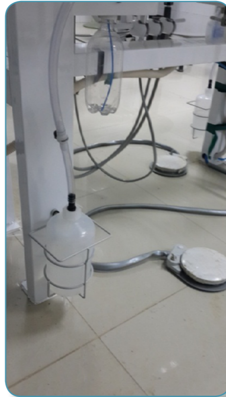
Installation of STU-DENT Duo workbenches / Connection to autonomous water supply
